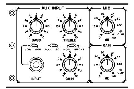
**Bass EQ:** Passive equaliser control, which can be set to provide up to 15dB of bass boost at 40Hz.
