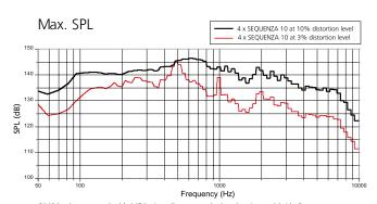
RMS levels measured with MF in 4 m distane, recalculated to 1 m, with Lb. Gruppen FP 1000 $\infty$ . Power supply 230 $\prime$ .
