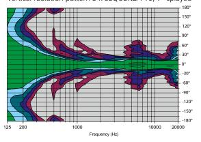
RMS levels measured with MFat 4 m distance with up to 50 % disortion level, recalculated to 1 m.Level values calculated for 4 x SEQUENZA, atual levels depend upon connection impedance and power supply.
