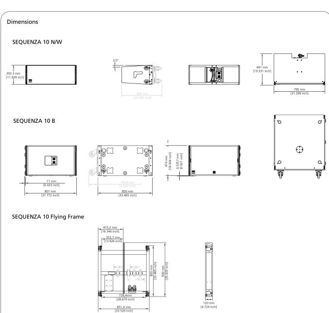
Weight of SEQUENZA 10 Flying Frame: 46 kg. Transport Cover with castors and the Groundstack Kit (grey) are optional accessories
